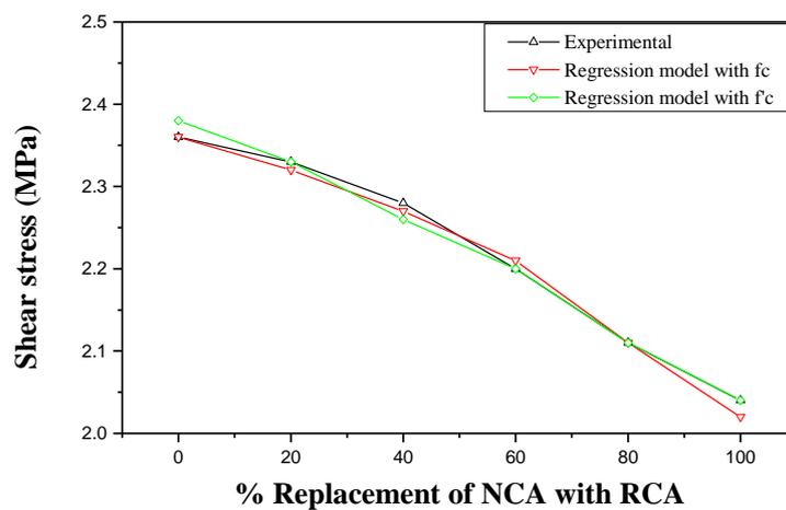
Fig 5: Variation of Shear stress with the replacement of NCA with RCA
