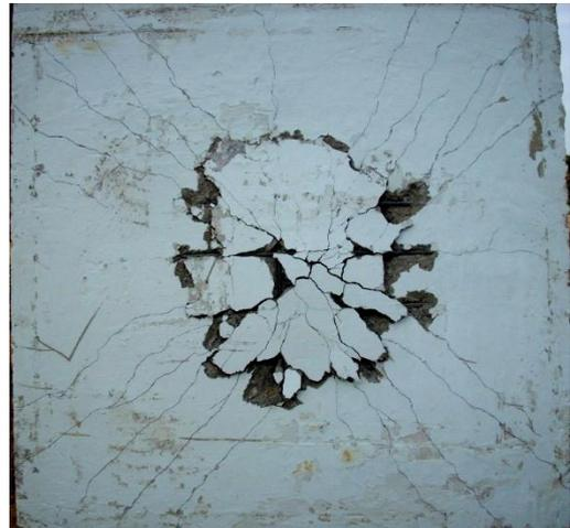
Fig 4: Typical bottom view of failure RCAC slab specimen
