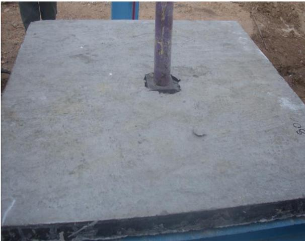
Fig 3: Typical top view of failure RCAC slab specimen
