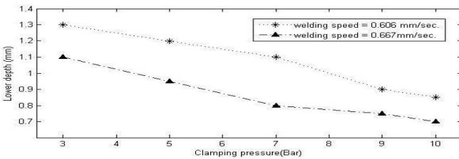
Fig. No.18: Lower depth (mm) versus Clamping pressure (Bar) of 2<sup>nd</sup> set
