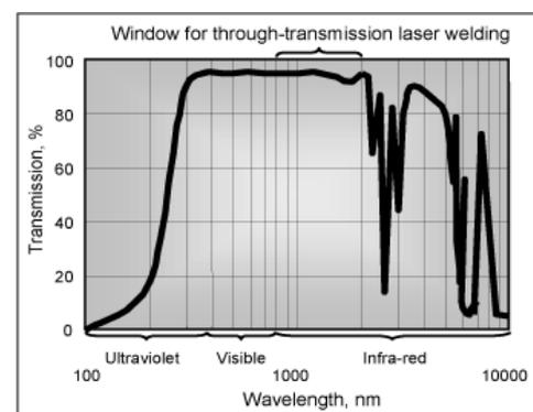
Fig.1. Absorption spectrum of a typical polymer[4]
