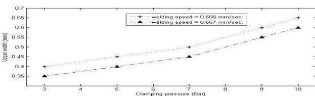
Fig. No.20 : Upper Width (mm) versus Clamping pressure (Bar) of 2<sup>nd</sup> set
