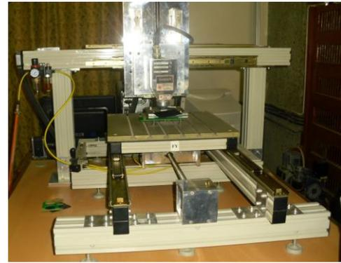
Fig. no.4: Laser CNC machine
