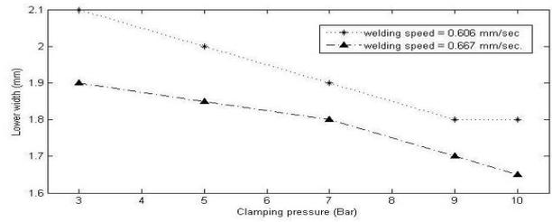
Fig. No.21 : Lower Width (mm) versus Clamping pressure (Bar) of 1<sup>st</sup> set
