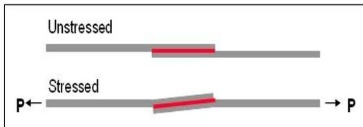
Figure 3: Schematic illustration (side view) of single lap joint before and after application of tensile stress [6].
