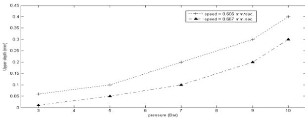
Fig. No.16: Upper depth (mm) versus Clamping pressure (Bar) of 2<sup>nd</sup> set
