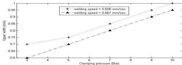
Fig. No.19: Upper Width (mm) versus Clamping pressure (Bar) of 1<sup>st</sup> set
