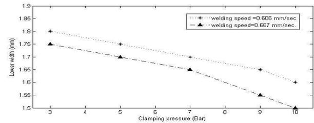
Fig. No.22 : Lower Width (mm) versus Clamping pressure (Bar) of 2<sup>nd</sup> set
