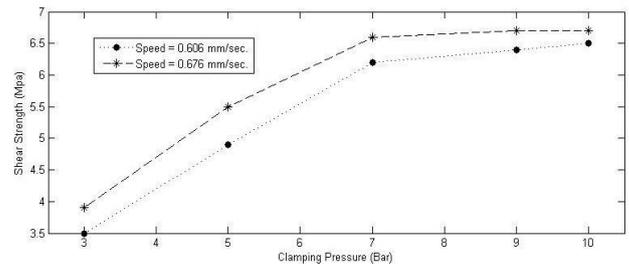
Fig. No.14: Shear strength (Mpa) versus Clamping pressure (Bar) of the 2<sup>nd</sup> set
