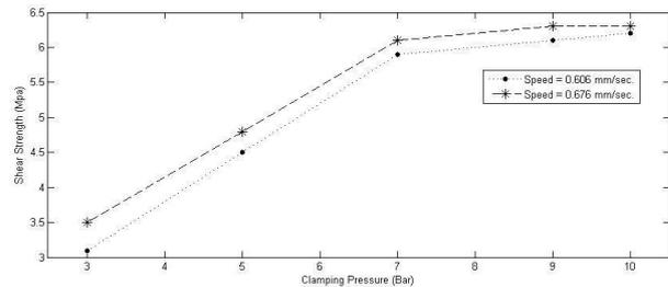
Fig. No.13: Shear strength (Mpa) versus Clamping pressure (Bar) of the 1<sup>st</sup> set
