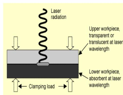
Fig.2. Through-transmission laser welding - cross-section through the welding process [4]
