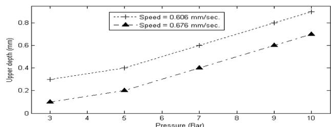
Fig. No.15: Upper depth (mm) versus Clamping pressure (Bar) of 1<sup>st</sup> set
