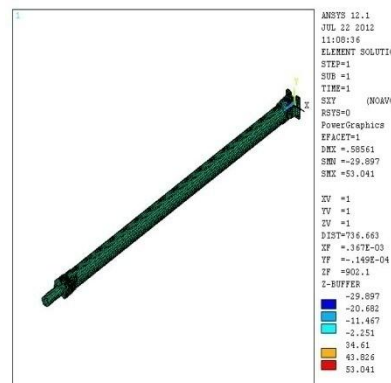
Fig 16: Steel shaft torsional analysis
