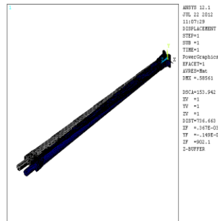
Fig 14: Steel shaft deformation results
