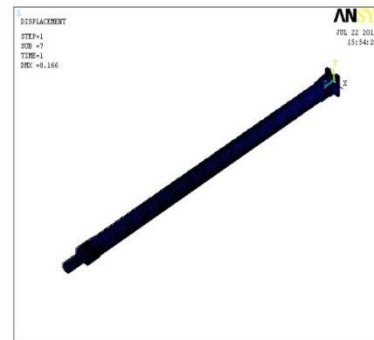
Fig 15: Kevlar/Epoxy drive shaft deformation results
