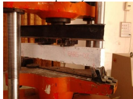
Figure 1: Flexural test setup
