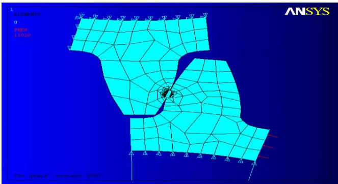
Figure 5 FEM Model of the gear tooth pair in contact
