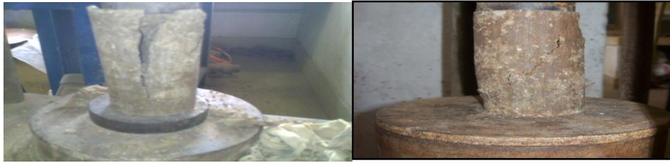
Figure 1: UCS Test - specimens crushed to total failure
