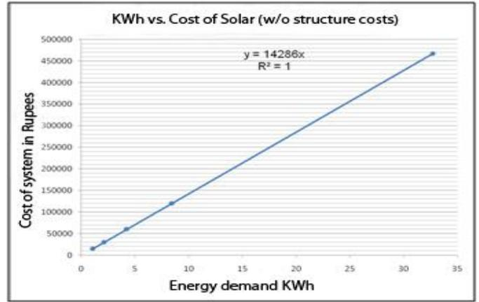
The graph shows a linear relationship between the energy demand and cost of the solar system (excluding the structure cost). Graph represented by the linear equation  $y = 14286x$ .
