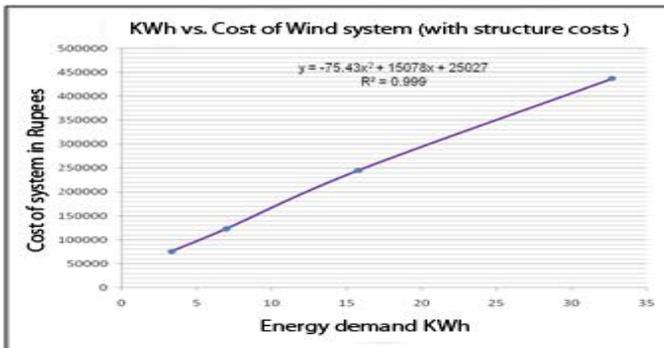
The graph shows a non linear relationship between the Energy demand and cost of the wind system (with structure cost). Graph represented by non linear equation  $y=75.43x^2+15078x+25027$  with a Correlation coefficient of  $R^2=0.999$
