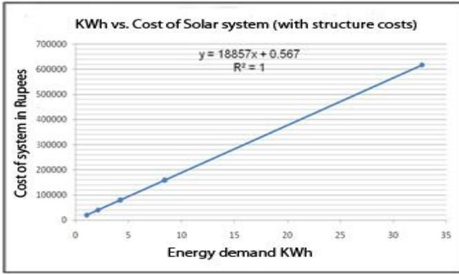
The above graph shows a linear relationship between the Energy demand and cost of the solar system (with structure cost). Graph represented by linear equation  $y=18857x+0.567$
