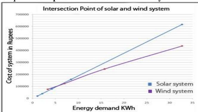
Graph #3 & Graph #4 were overlapped (i.e. energy demand vs. cost of solar system and wind system
