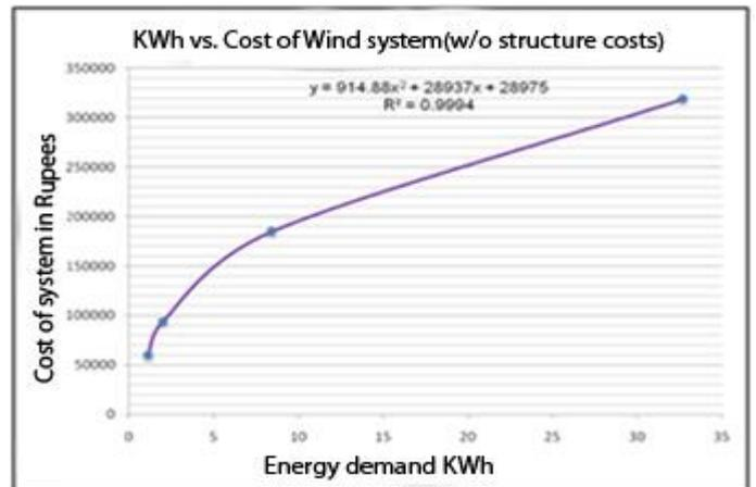
The above graph shows nonlinear relation between the energy demand and wind system cost (excluding the structure costs). Graph represented by the polynomial equation  $y = 914.88x^2 + 28937x + 28975$  with a correlation coefficient of  $R^2 = 0.9994$ .
