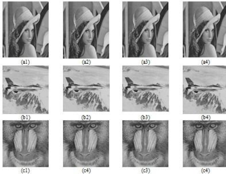
Figure 11. Obtained shadows from (2, 4) -threshold user-friendly image sharing scheme with four different primes \{p_1, p_2, p_3, p_4\} = \{17, 61, 131, 251\}
