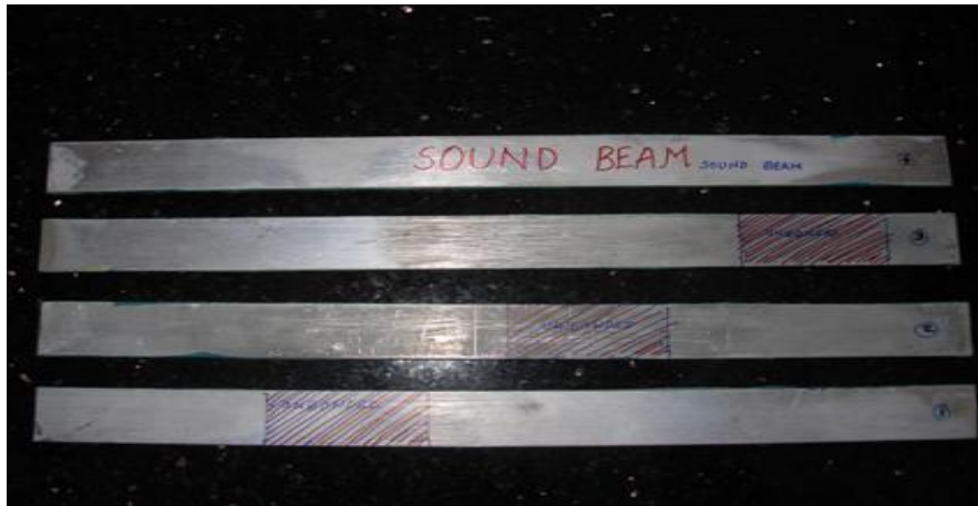
Fig 3. Two layered metallic beam specimens with 50 mm delaminations
