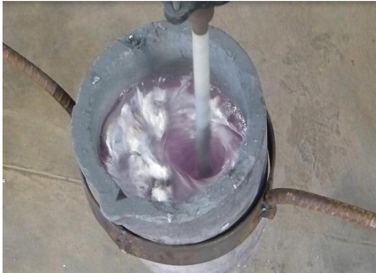
Fig. 1. The molten metal was stirred to create a vortex
