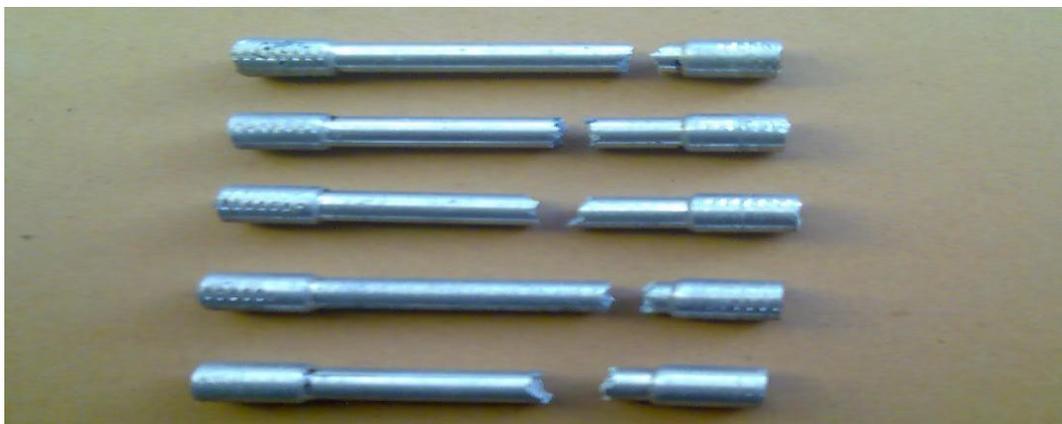
Fig. 2. Composite specimens after tensile test
