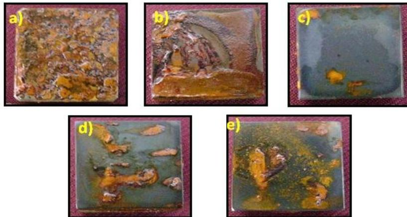
Figure 5. Surface pictures of samples after 21h exposed to rich chloride fog. a) Untreated, b) nitrided, and post-oxidized during c) 15, d) 30 and e) 60 minutes.
