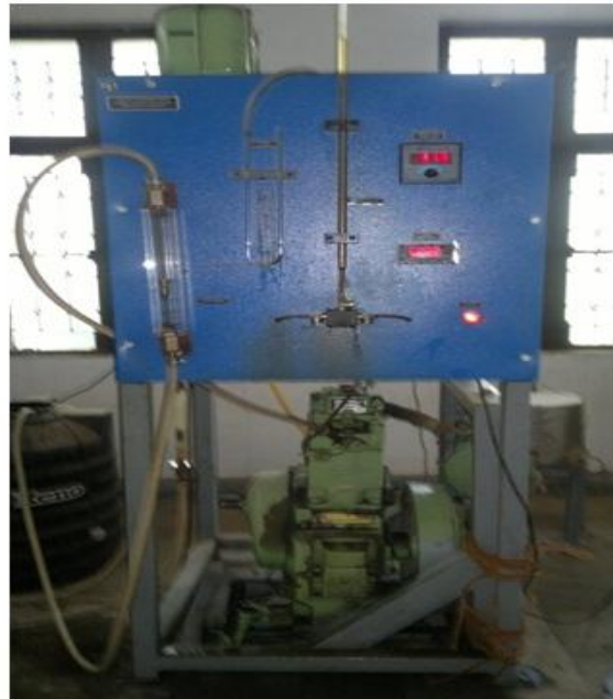
Figure 1: Single Cylinder Four Stroke Diesel (CI) Engine Experimental Setup
