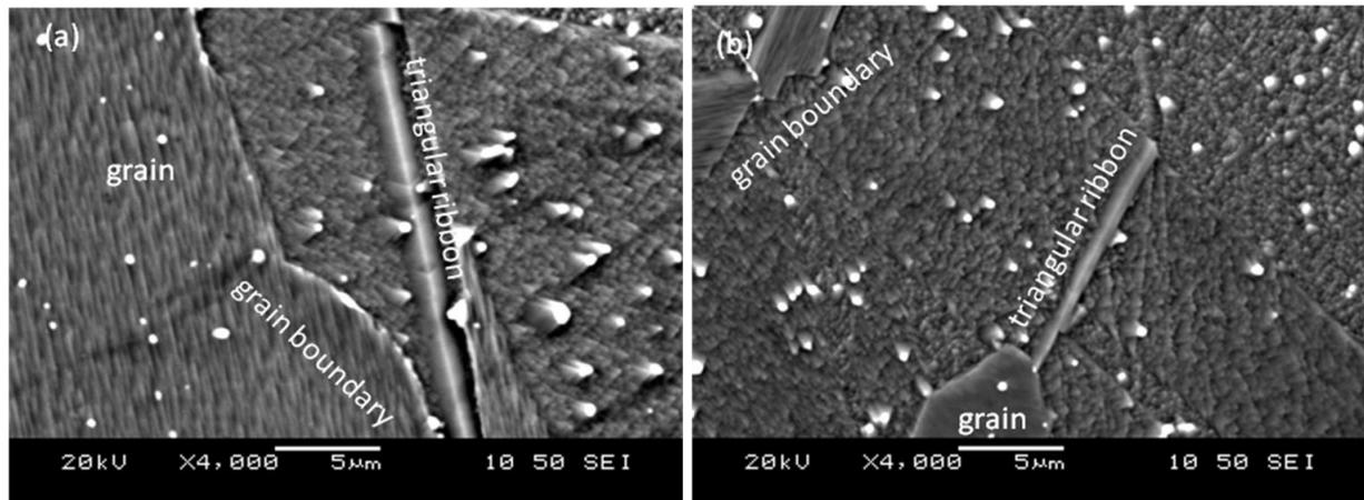
Figure 2: Scanning electron micrographs of Inconel 600 specimens showing short triangular ribbon-type slip bands fatigued at (a) 500MPa and  $7 \times 10^5$  cycles, (b) 550MPa and  $3 \times 10^5$  cycles.
