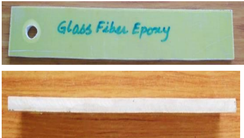
Fig. 6.1 Glass Fiber Epoxy Test Specimen
