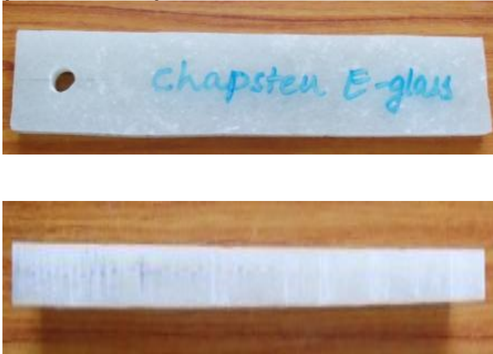
Fig. 6.4 Chapsten E-Glass Epoxy Test Specimen
