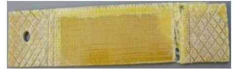
5.7 Chapsten E-Glass Epoxy Specimen after Tensile Test
