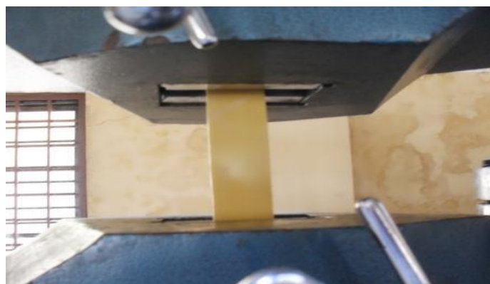
Fig. 5.4 Tensile Test in Process
