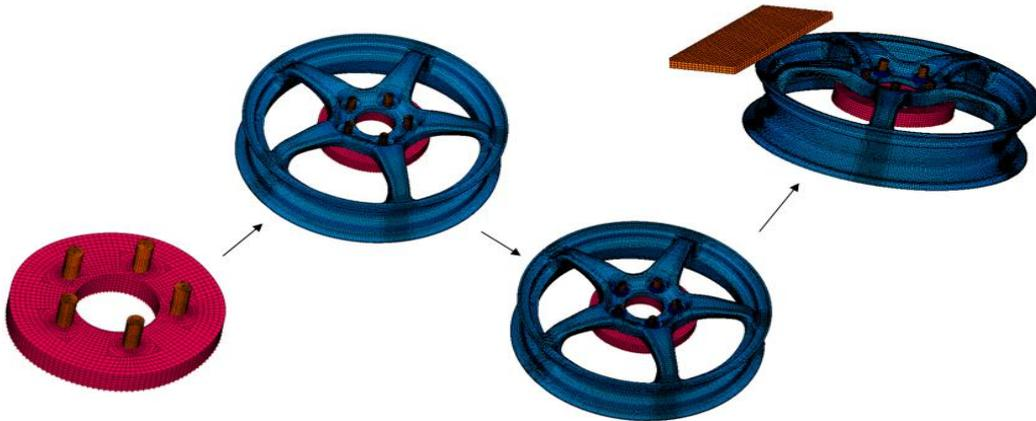
**Figure 4.** Finite element model of the Wheel Assembly with Striker
