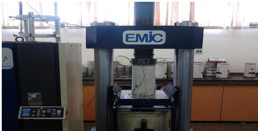
Fig. 2.2 Compressive Strength Test, conducted at the Laboratory of Concrete Department of Technical Support and Control of Furnas Centrais Elétricas S.A. in Goiânia-GOÍÁS
