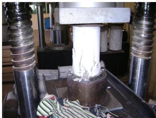
Fig. 2.1 Compressive Strength Test, conducted at the Laboratory of Building Materials Company Carlos Campos Consultoria and Construções Ltda. in Goiânia-GOÍAS
