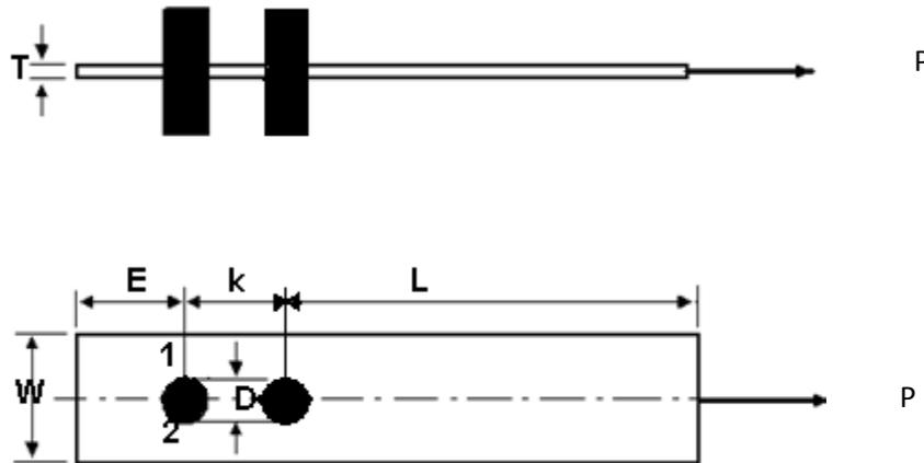
Fig. 1. Geometry of the specimen
