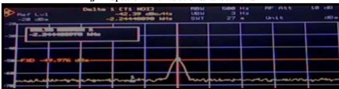
Fig. 18 Spectrum when value of C/N_0=36.71\text{dBc/Hz}
