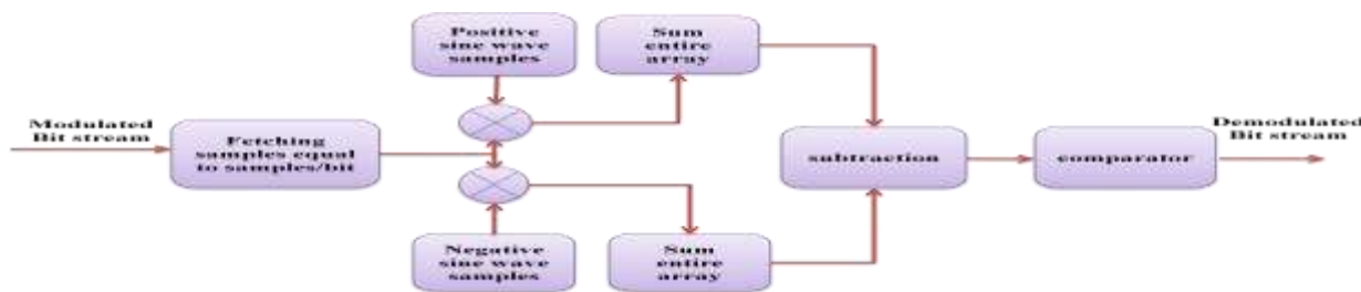
Fig.2. Principal of BPSK Demodulation[2]
