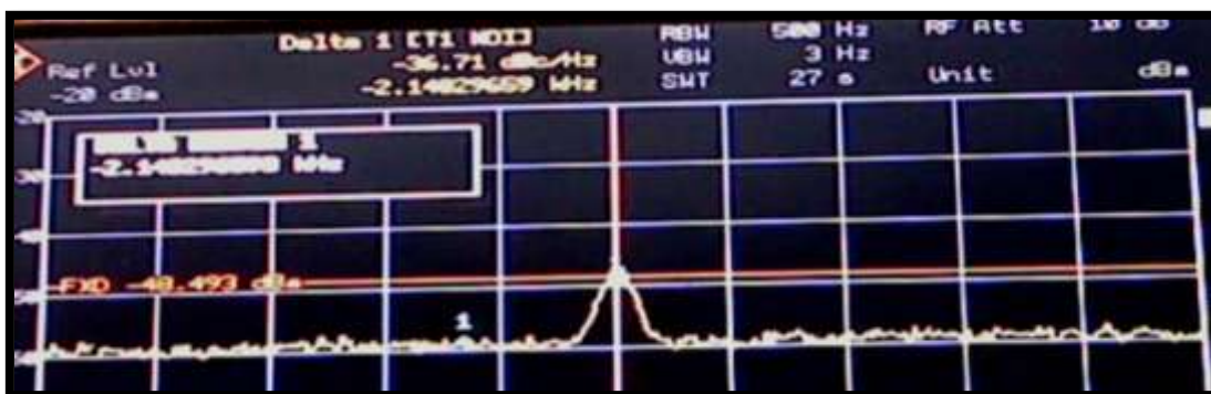
Fig.16 Spectrum when value of C/N_0=36.71\text{dBc/Hz}
