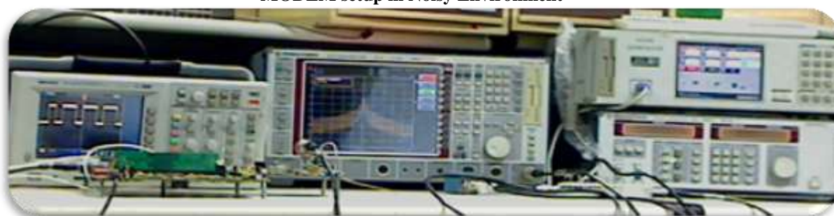
Fig. 23 Experimental setup for BPSK MODEM setup in Noisy Environment
