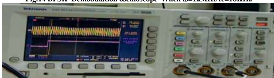
Fig.15 Experimental set up for BPSK Demodulation When f_s=12\text{MHz} f_c=48\text{KHz}
