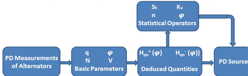
Fig.1 (b) Block diagram of discharge analysis for ( $\phi$ - $n$ )
