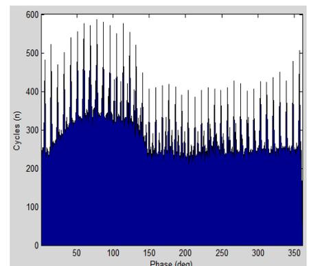
Fig.5(c).Phase plot ( $\varphi$ -n) of corona discharge
