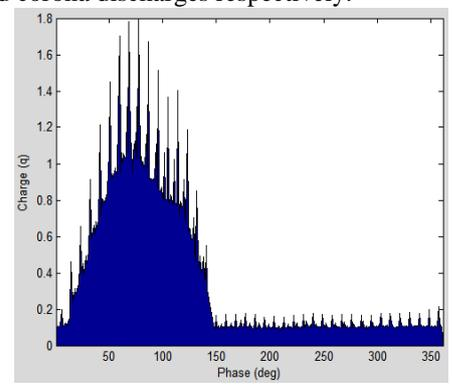
Fig.3(c). Phase plot (φ-q) of corona discharge
