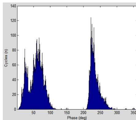
Fig.5(b).Phase plot ( $\varphi$ -n) of surface discharge
