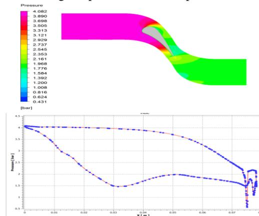
Fig.16 Contours of static Pressure at mid plane
