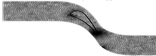
Fig.15 Turbine Blade Meshing
