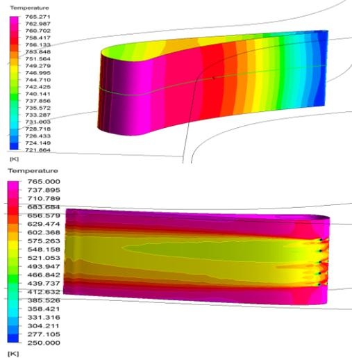
Fig.18 Temperature contours-With and without showerhead cooling holes
