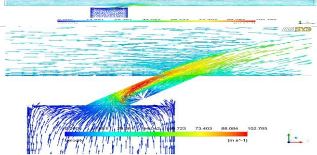
Fig.8 Velocity vectors contours of film cooling
