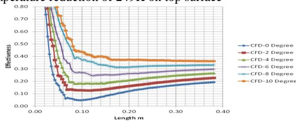
Fig. 13 Comparison of Effectiveness contours of film cooling-0-10<sup>0</sup>
