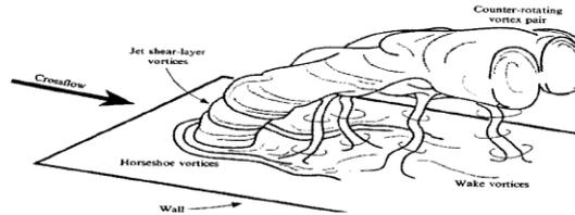
Fig.4 Flat plate Film cooling
