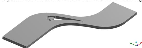
Fig.17 C3X vane with shower head cooling Hole
