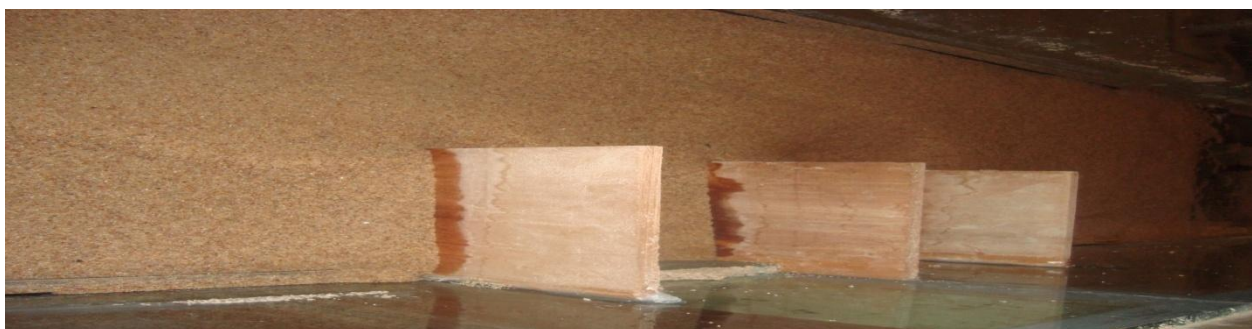
Plate (1): Front view of the groynes
