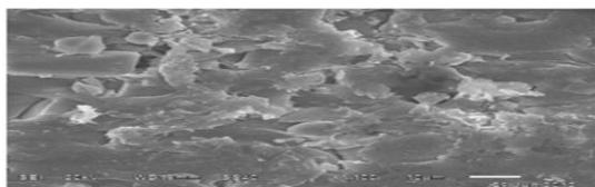
**Fig 4.10 SEM: PPS/40%GF/0% nano-CaCO<sub>3</sub>**
