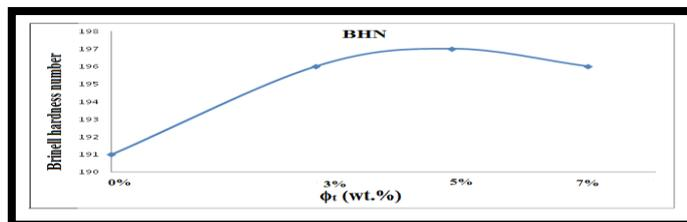
**Fig.4.9 Effect of weight fraction of Nano-CaCO<sub>3</sub> ( $\phi_f$ ) on Brinell hardness number (BHN)**
