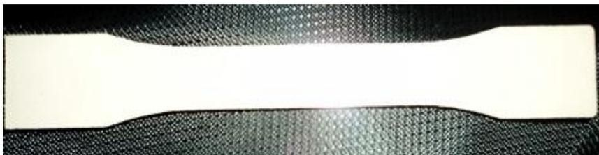
Fig: Tensile specimen As per ASTM D638
