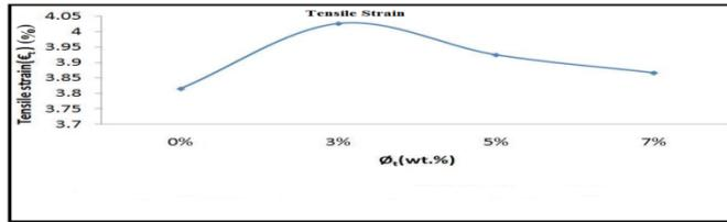
**Fig 1.2: Effect of weight fraction of Nano-CaCO<sub>3</sub> ( $\phi_f$ ) on Tensile Strain ( $\epsilon_t$ )**
