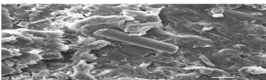
**Fig 4.12 SEM: PPS/40%GF/5% nano-CaCO<sub>3</sub>**
