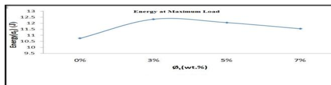
**Fig:1.4 Effect of weight fraction of Nano-CaCO<sub>3</sub> ( $\phi_f$ ) on Energy( $\sigma_E$ )**
