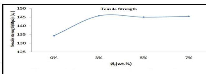
**Fig 1.1: Effect of weight fraction of Nano-CaCO<sub>3</sub> ( $\phi_f$ ) on tensile strength ( $\sigma_t$ )**
