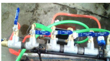
Figure 2.3: Flow distribution system
