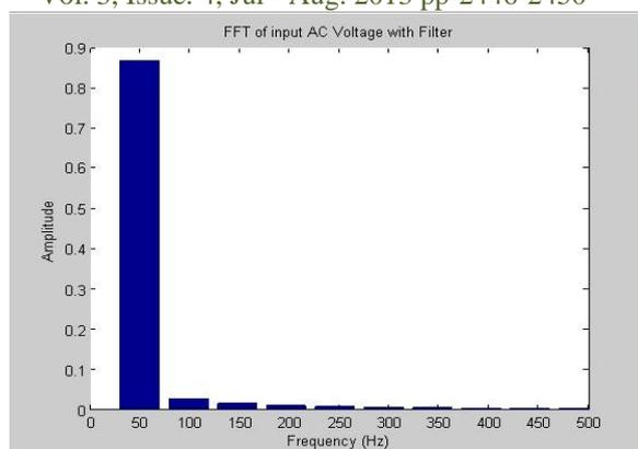
Fig.6. FFT of input AC Voltage with Filter
