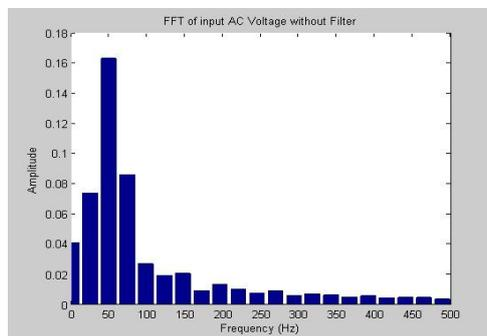
Fig.4. FFT of input AC Voltage without Filter
