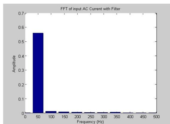
Fig.7. FFT of input AC Current with Filter
