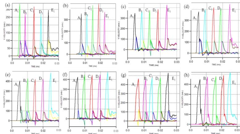
Figure 3 Collision speed of composite pipe under different gap (a)0.3mm gap (b)0.4mm gap (c)0.5mm gap (c)0.6mm gap (e)0.7mm gap (f)0.8mm gap (g)0.9mm gap (h)1mm gap
