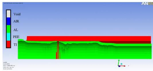
Figure 4 Situation of rupture of flyer tube
