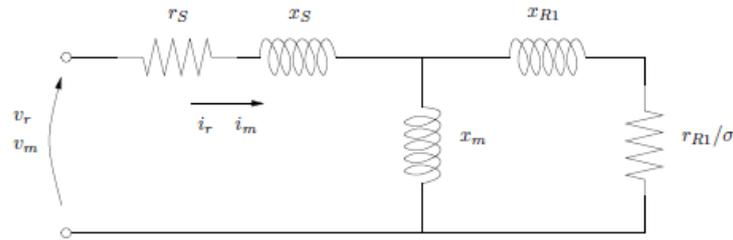
Figure 2. Simplified electrical circuit for single cage IM.
