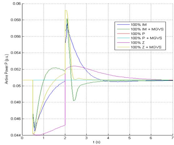
Figure 6. Comparison of Active Power at Bus 15 for Case Study 1.
