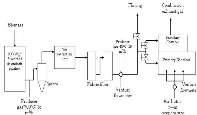
Fig.4 Schematic diagram of experimental apparatuses
