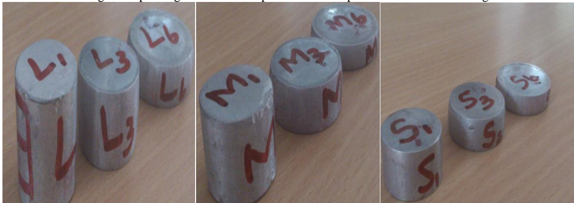
Fig.4. Deformed specimen for various aspect ratios -1.0, 0.8 and 0.6
