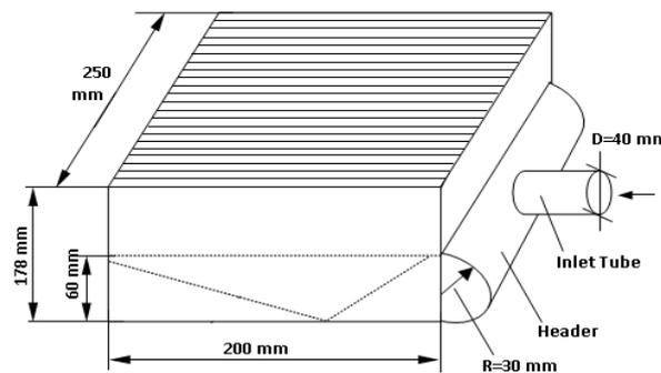
Plate -fin heat exchanger
