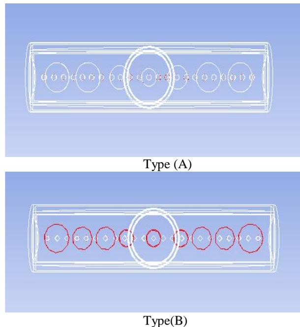
Fig.2 Schematic model of modified header configurations with type(A) and type(B)
