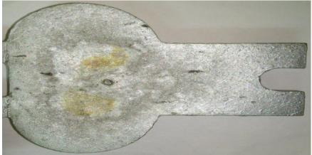
Fig. 15. casting without feeder shows defect
