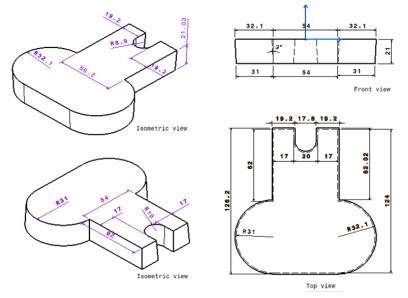
Fig.1. wooden pattern with allowances for casting
