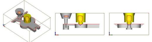
Fig. 7. partial shifted position of hotspot with the application of feeder
