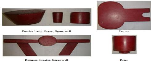
Fig. 13. wooden rigging system with pattern
