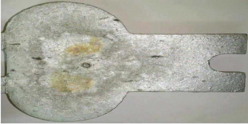
Fig. 15. casting without feeder shows defect
