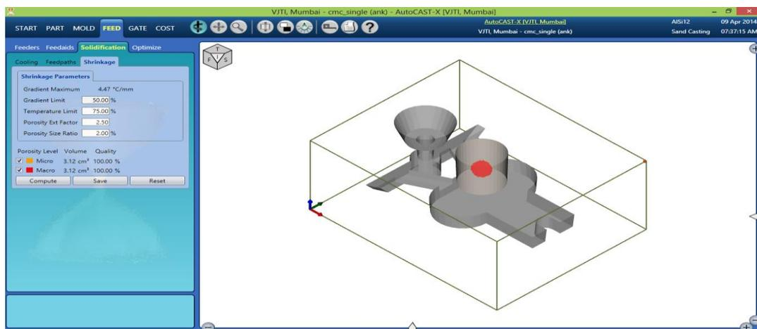
Fig. 11. shrinkage porosity as seen in 3d, side view and front view (macro-red, micro-orange)
