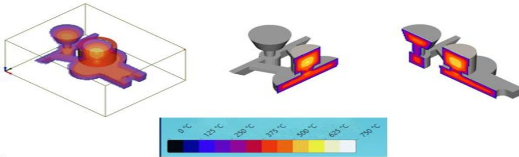
Fig. 9. cooling simulation of casting in 3D
