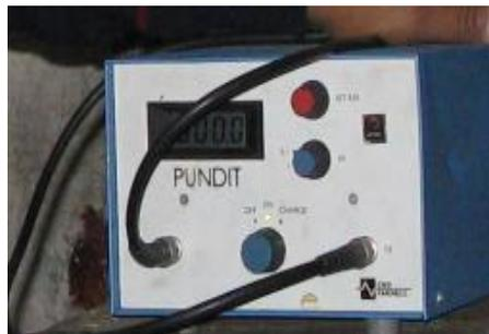
Figure 3: Portable Ultrasound Non destructive Digital Indicator Tester Equipment (PUNDIT)
