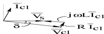
Figure (2) : phasor diagram for reactive power flow from the DSTATCOM .
