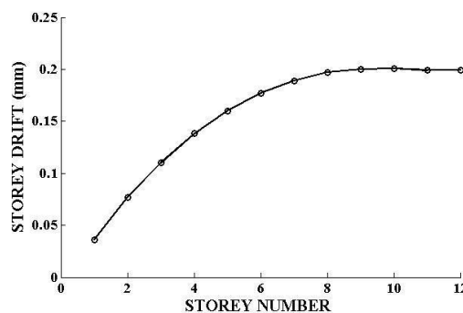
Figure 9: Storey drifts on shear walls
