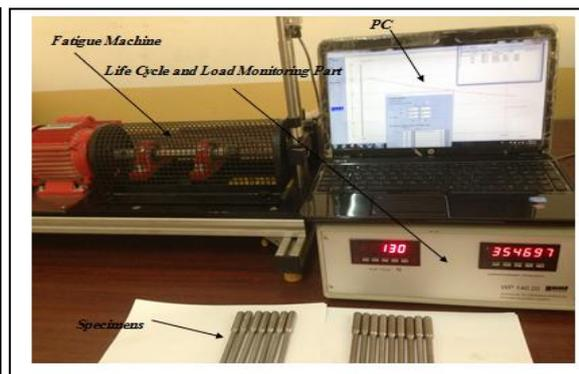
Fig. 3 Fatigue testing machine WP 140
