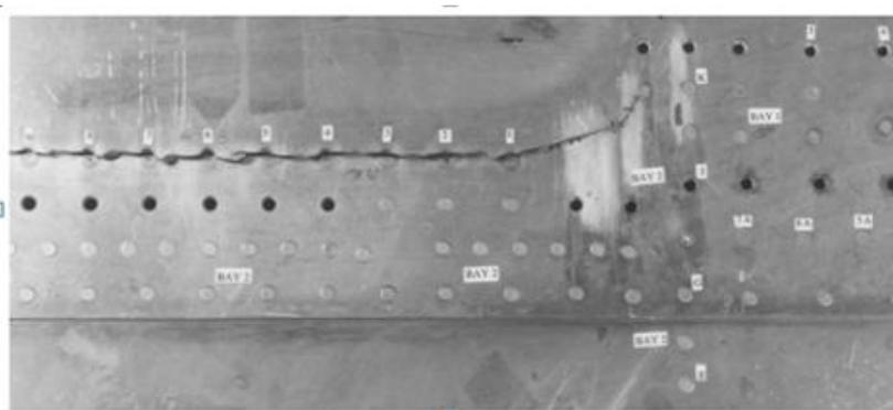
Fig.1. Larger crack formed by the link-up of fatigue cracks at adjacent rivets
