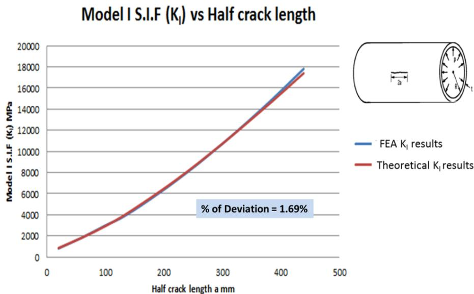
Fig.7: variation of theoretical and FEA values of S.I.F Vs crack length in Pressurized cylinder
