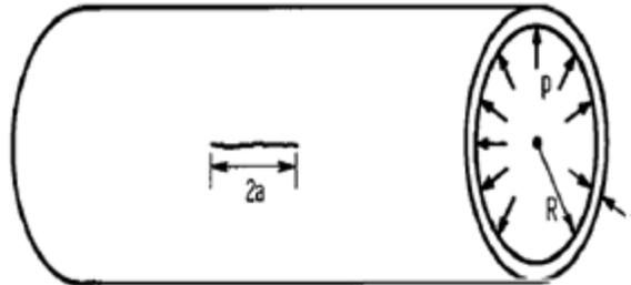
Fig.6: Longitudinal crack in internally pressurized cylinder
