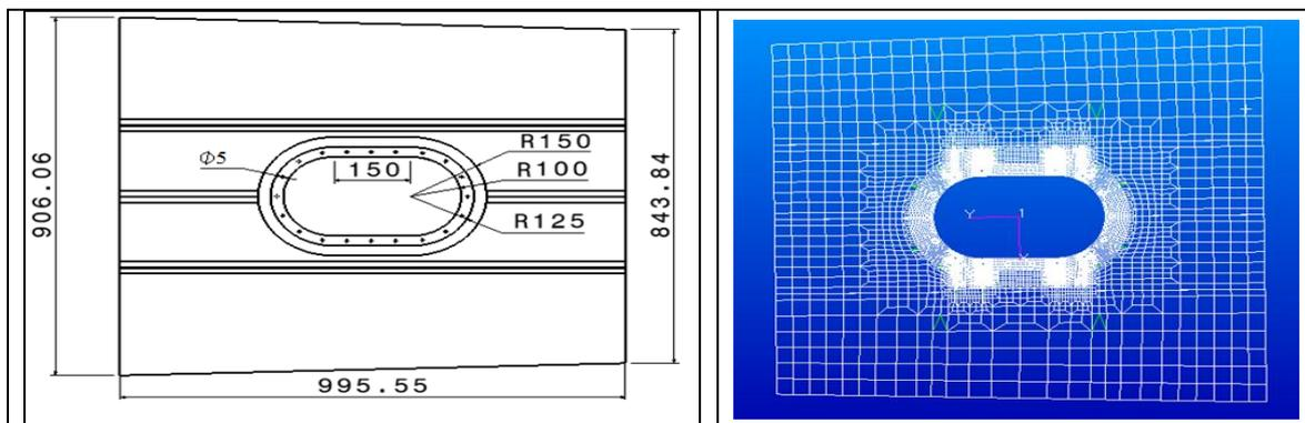
Fig.3.6 Geometry of local model; FE Model of local model
