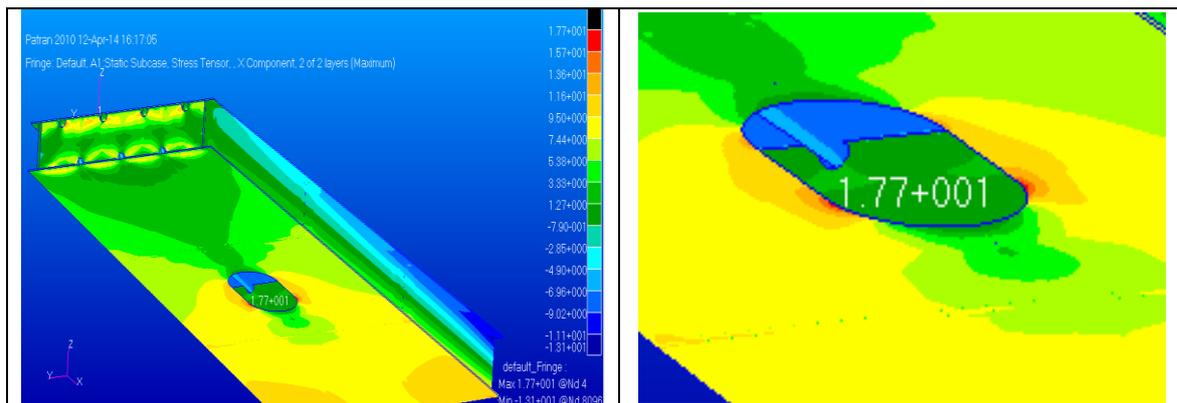
Fig.3.5 Maximum stress in wing box (global model)
