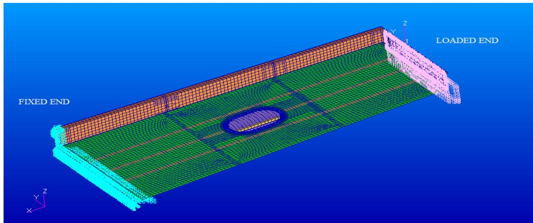
Fig.3.4 Boundary conditions of wing box (global model)
