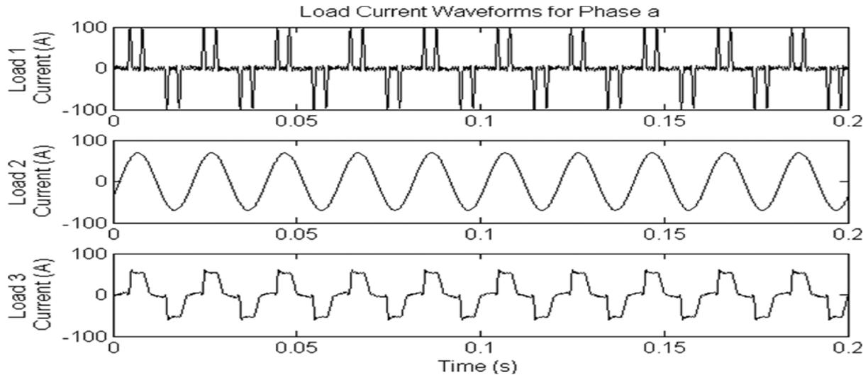
Fig. 9. Per-phase currents drawn by loads 1, 2, and 3.
