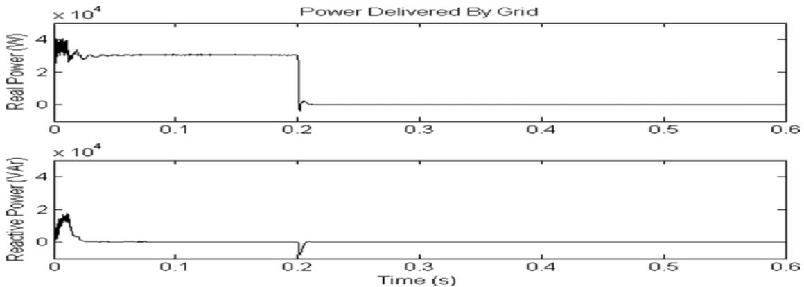
Fig. 20. Real (top) and reactive (bottom) power delivered by the grid
