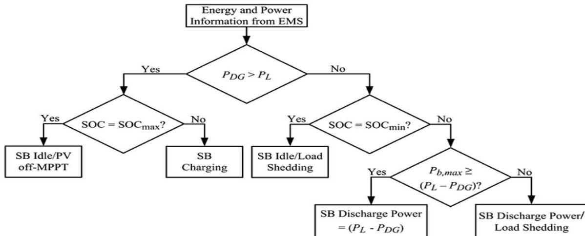
Fig. 3. Operation of the SB during islanded operation
