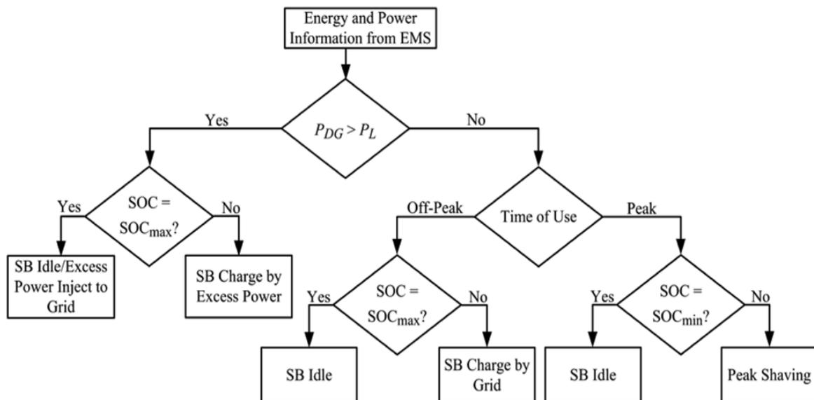
Fig. 2. Operation of the SB during grid-connected operation
