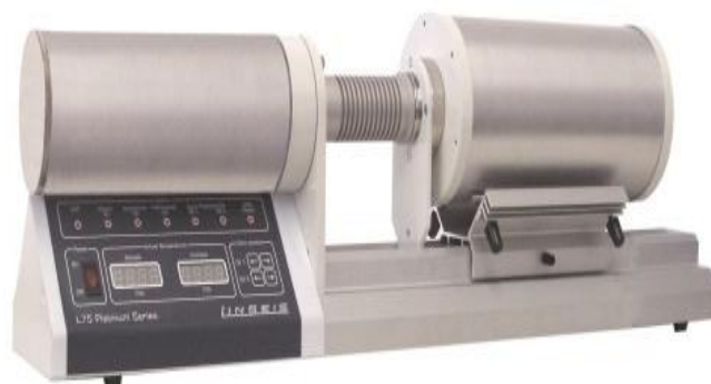
Fig 3.1- Linessis 75 Platinum Horizontal Dilatometer
