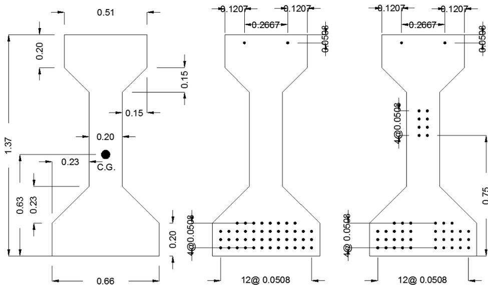
Fig. 2 Beam details of Type IV AASHTO beam
