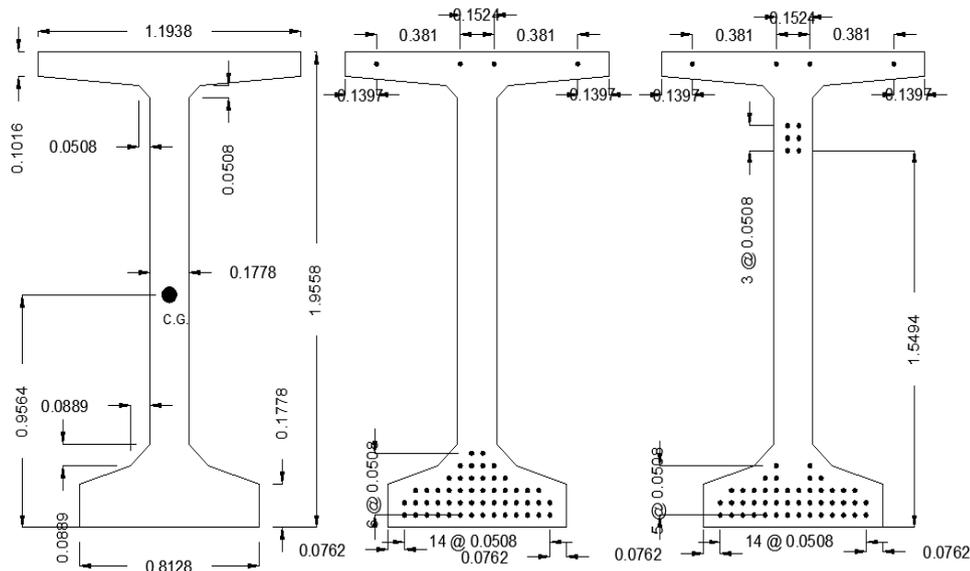
Fig. 1 Beam details of 77in. PCI Bulb Tee
