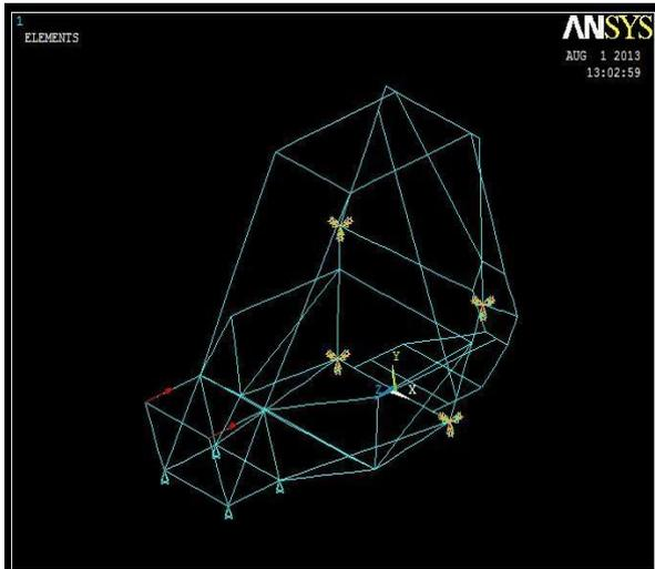
Figure 4. Frontal impact load application
