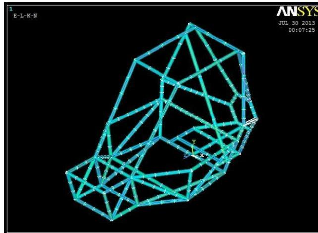
Figure 3. Meshed model with element shape
