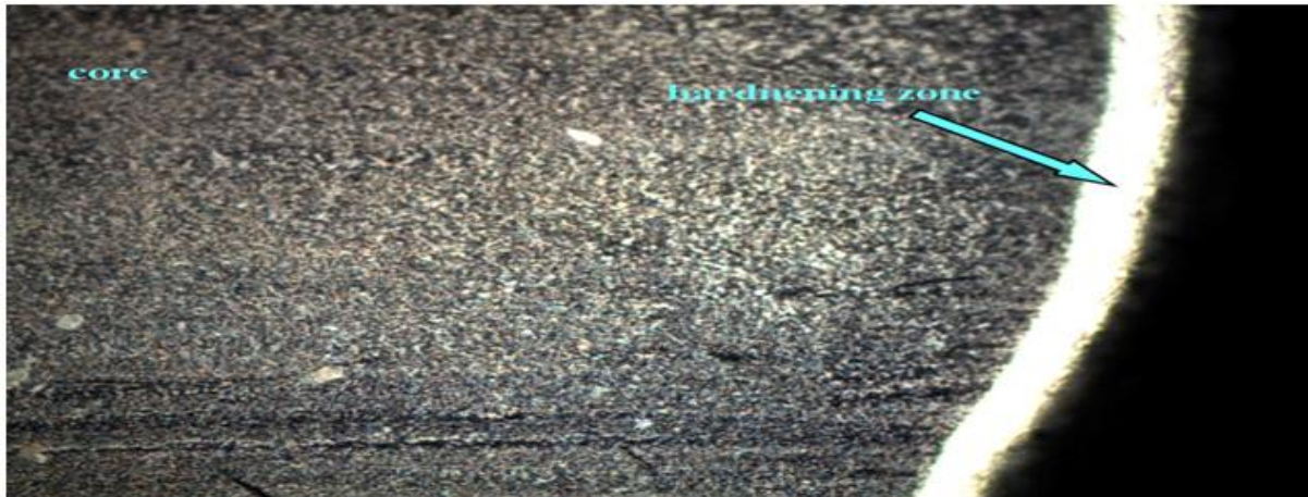
Fig. 3.5 Optical Photo Micrograph of Induction Hardened Steel Specimen Magnified 20X
