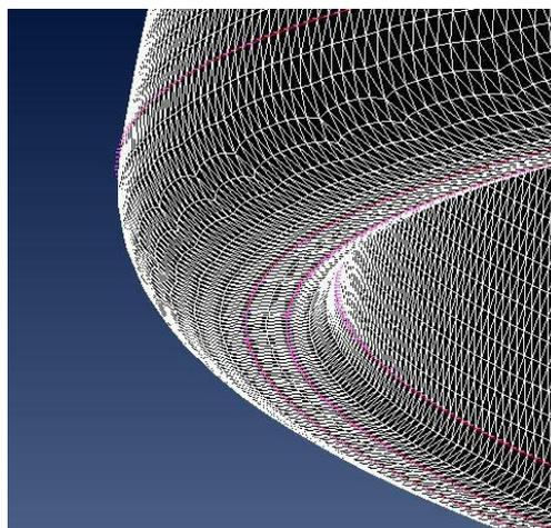
**Fig 4** Surface mesh containing tetrahedral mesh only
