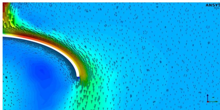
Fig 8 Pressure contours the streamlines flow, and wake
