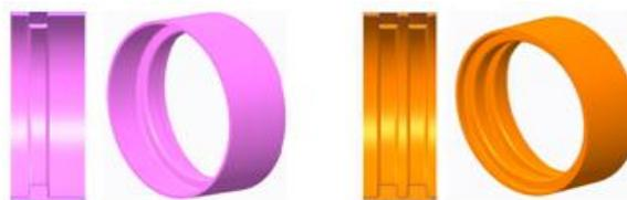
**Fig 6:** Oil cavity 3D geometry of Turbocharger under study
