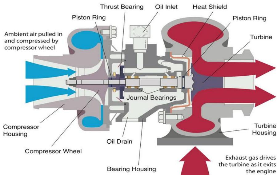
**Fig 1:** Components in Turbocharger and Oil Flow Path
