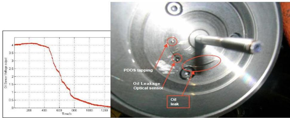
**Fig 5:** Turbocharger Oil Leakage Detection Method
