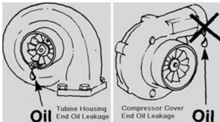
Fig 4: Leakage at Turbine housing & Compressor Cover
