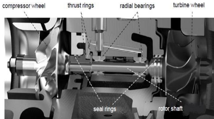
Fig 2: Seal Rings Position in Turbocharger
