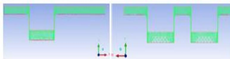
**Fig 7:** Mesh of one & two piston seal ring cavity
