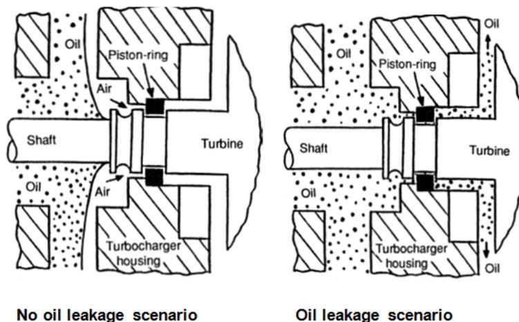
Fig 3: Turbine end no oil leakage & oil leakage scenario
