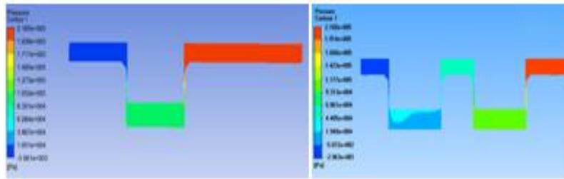
Fig 9 CFD results for 30 psi pressure at 30 degree C with Single & Double seal
