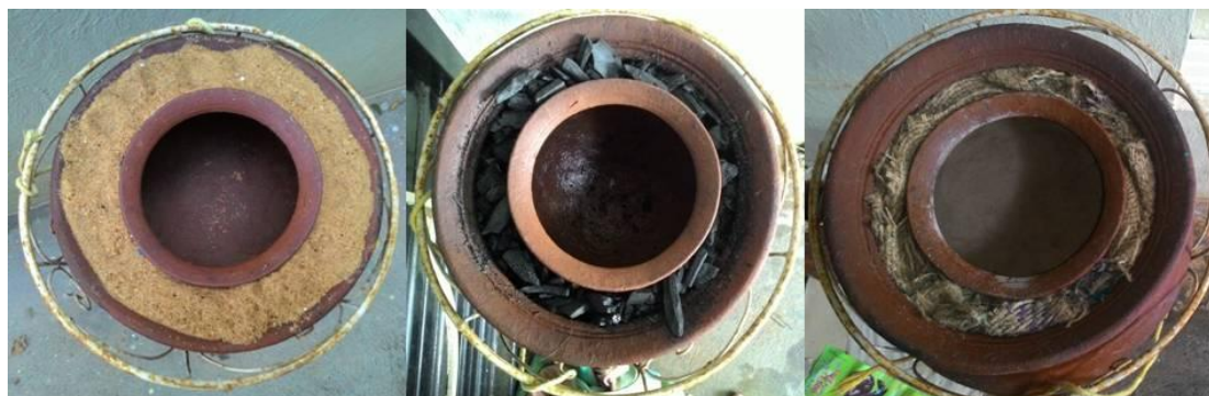
Figure 2: Zeer Pot filled with (a) Sand (b) Charcoal (c) Gunny Cloth
