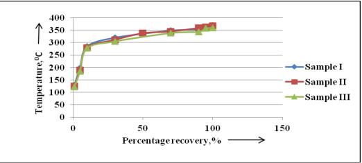
Figure 2: Distillation curve of sample I, II & III
