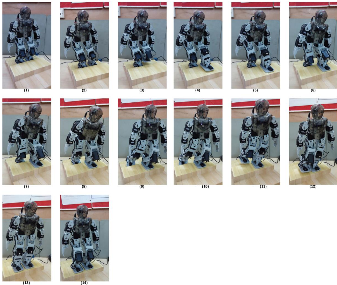
Fig. 10. Various poses for step up stairs implemented on BIOLOID Humanoid
