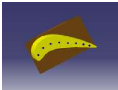
Fig 2.1. Top View for Profile of gas turbine rotor blade with cooling pipes
