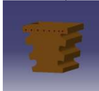
Fig.2.2. Fir root of rotor blade
