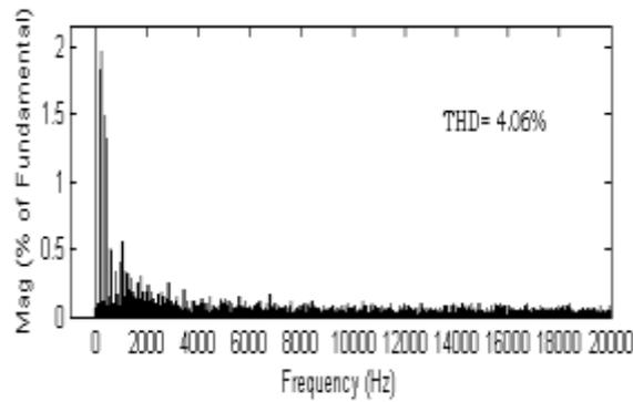
Fig. 27 Harmonic spectra of stator current in proposed 24 - Sector algorithm based vector controlled induction motor drive
