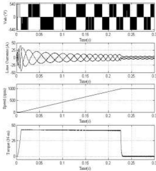
Fig. 13 starting transients of 6 - Sector algorithm vector control algorithm based induction motor drive
