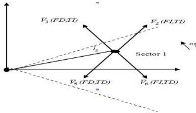
**Fig. 4** selection of suitable voltage space vector in sector I ( $-30^0$  to  $30^0$ )
