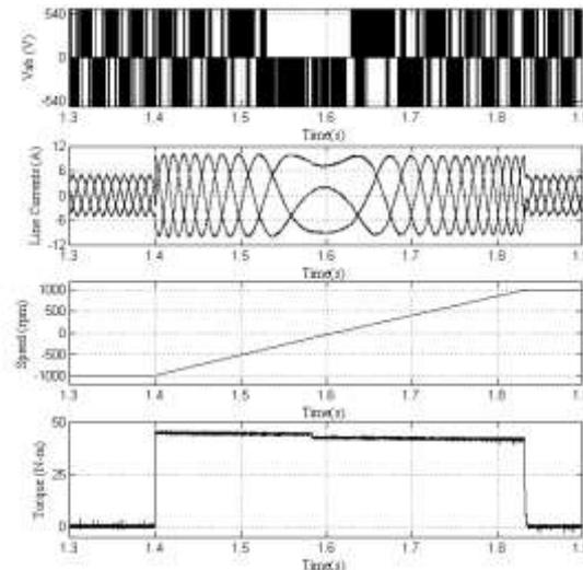
**Fig. 30** Transients during the speed reversal (from -1000 rpm to +1000 rpm) for proposed 24 - Sector algorithm based vector controlled induction motor drive
