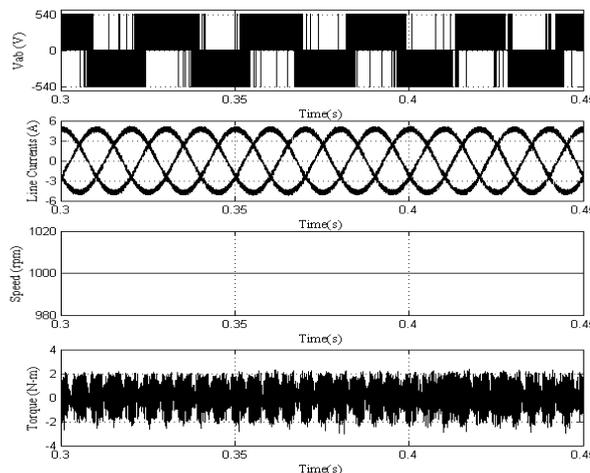
**Fig. 8** steady state plots of classical vector control algorithm based induction motor drive
