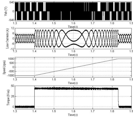
Fig. 12 Transients during the speed reversal (from -1000 rpm to +1000 rpm) for classical vector control algorithm based induction motor drive
