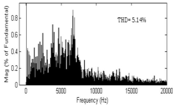
Fig. 15 Harmonic spectra of stator current in 6 - Sector algorithm vector control algorithm based induction motor drive
