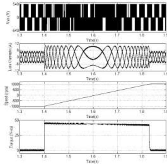
**Fig. 24** Transients during the speed reversal (from -1000 rpm to +1000 rpm) for proposed 12 - Sector algorithm based vector controlled induction motor drive
