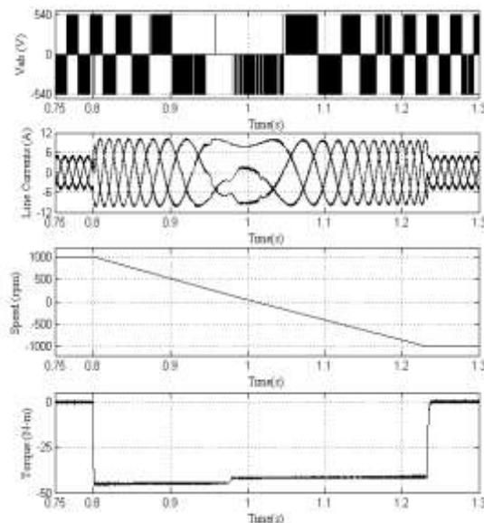
Fig. 17 Transients during the speed reversal (from +1000 rpm to -1000 rpm) for 6 - Sector algorithm vector control algorithm based induction motor drive
