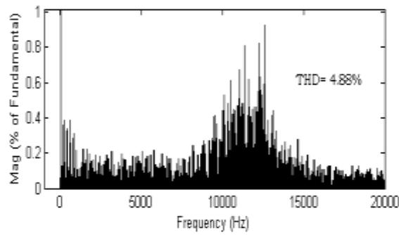
Fig. 21 Harmonic spectra of stator current in proposed 12 - Sector algorithm based vector controlled induction motor drive
