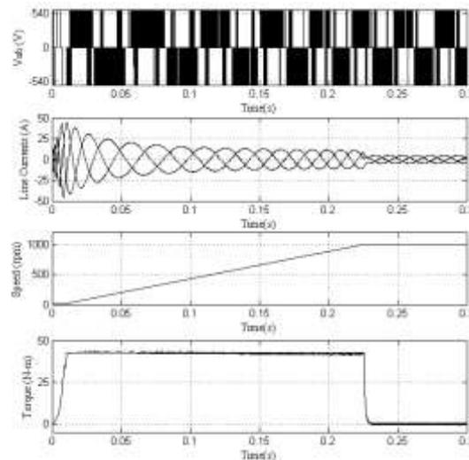
**Fig. 25** starting transients of proposed 24 - Sector algorithm based vector controlled induction motor drive
