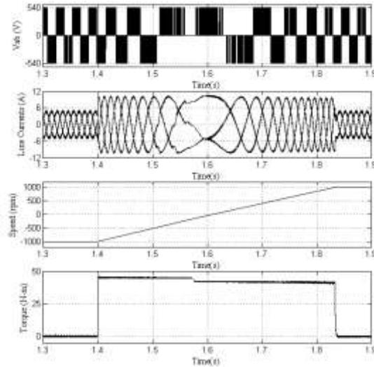
**Fig. 18** Transients during the speed reversal (from -1000 rpm to +1000 rpm) for 6 - Sector algorithm vector control algorithm based induction motor drive
