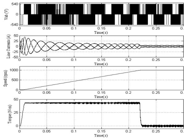
**Fig. 7** starting transients of classical vector control algorithm based induction motor drive
