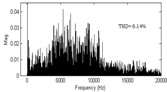
Fig. 9 Harmonic spectra of stator current in classical vector control algorithm
