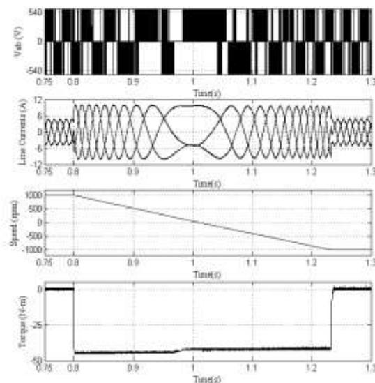
Fig. 29 Transients during the speed reversal (from +1000 rpm to -1000 rpm) for proposed 24 - Sector algorithm based vector controlled induction motor drive
