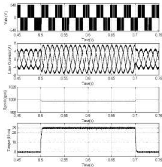
Fig. 16 Transients during the step change in load (a 25 N-m load is applied at 0.5 sec and removed at 0.7 sec) for 6 - Sector algorithm vector control algorithm based induction motor drive
