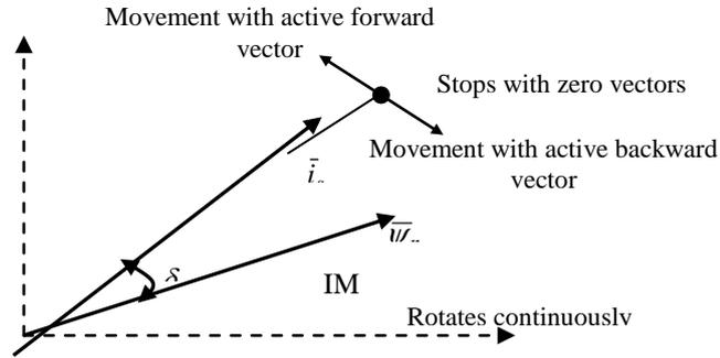
Fig. 1 movement of stator current vector under the influence of voltage vectors
