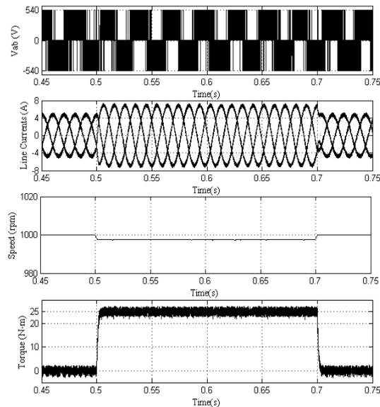
Fig. 10 Transients during the step change in load (a 25 N-m load is applied at 0.5 sec and removed at 0.7 sec) for classical vector control algorithm based induction motor drive
