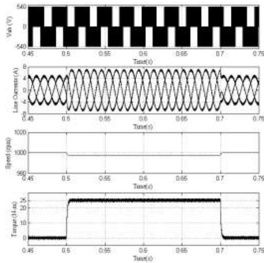
Fig. 22 Transients during the step change in load (a 25 N-m load is applied at 0.5 sec and removed at 0.7 sec) for proposed 12 - Sector algorithm based vector controlled induction motor drive
