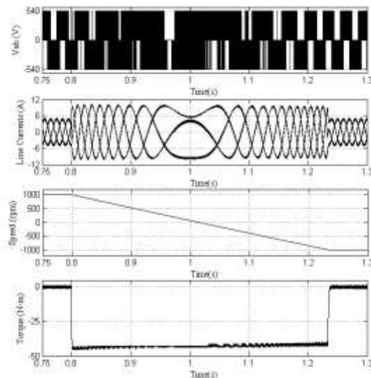
Fig. 23 Transients during the speed reversal (from +1000 rpm to -1000 rpm) for proposed 12 - Sector algorithm based vector controlled induction motor drive
