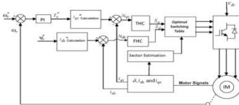
Fig. 2 Block diagram of proposed vector controlled induction motor drive
