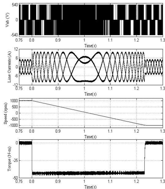
Fig. 11 Transients during the speed reversal (from +1000 rpm to -1000 rpm) for classical vector control algorithm based induction motor drive
