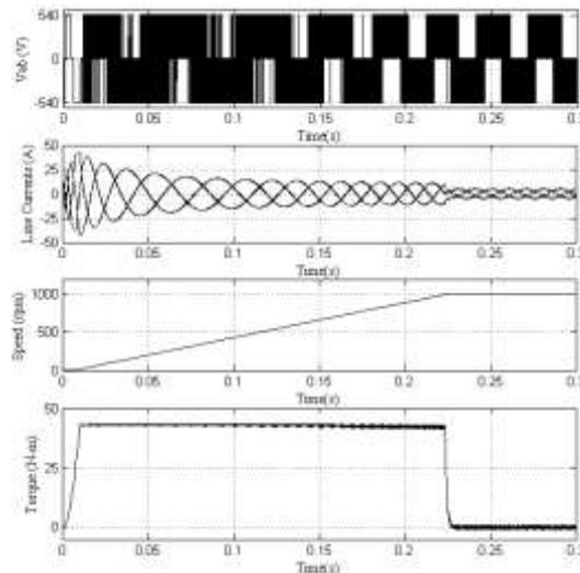
**Fig. 19** starting transients of proposed 12 - Sector algorithm based vector controlled induction motor drive
