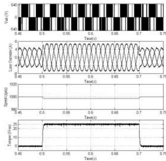
Fig. 28 Transients during the step change in load (a 25 N-m load is applied at 0.5 sec and removed at 0.7 sec) for proposed 24 - Sector algorithm based vector controlled induction motor drive
