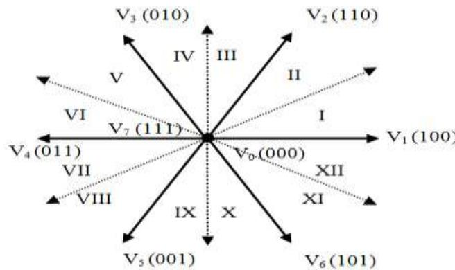
Fig. 5 Possible voltage space vectors for VSI in 12- sector based vector control algorithm
