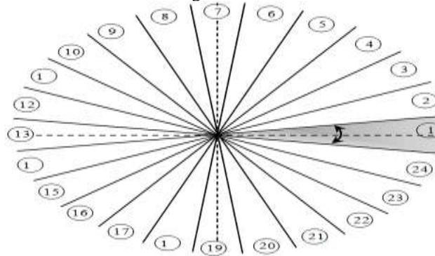
Fig. 6 Possible voltage space vectors for VSI in 24- sector based vector control algorithm
