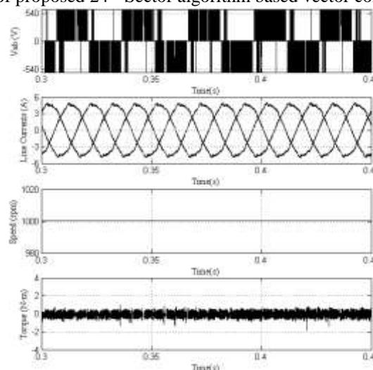
**Fig. 26** steady state plots of proposed 24 - Sector algorithm based vector controlled induction motor drive
