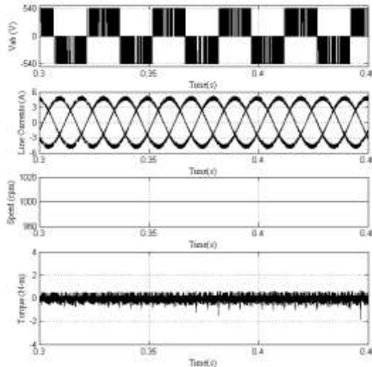
Fig. 14 steady state plots of 6 - Sector algorithm vector control algorithm based induction motor drive
