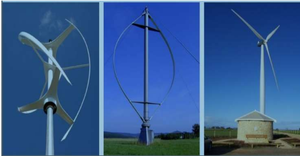
Fig. 1. Schematic of wind turbines: VAWT (left and center panels) and HAWT (right panel) [6,7].
